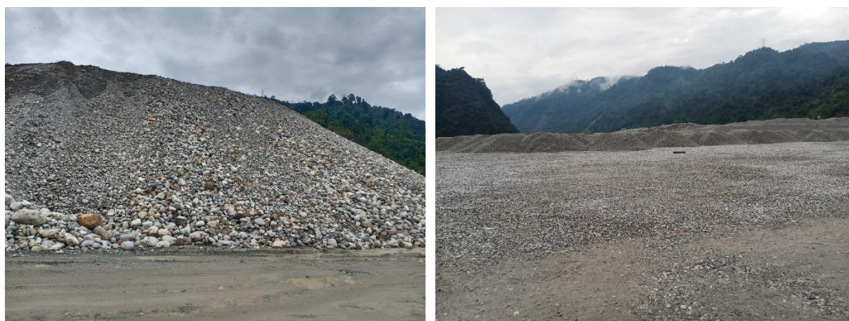
Figure 3. Stock of Toorsa riverbed sediments as construction material
